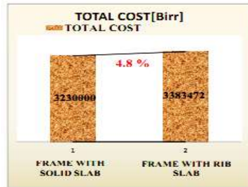
Figure 6. Total Cost Comparison of Frame
