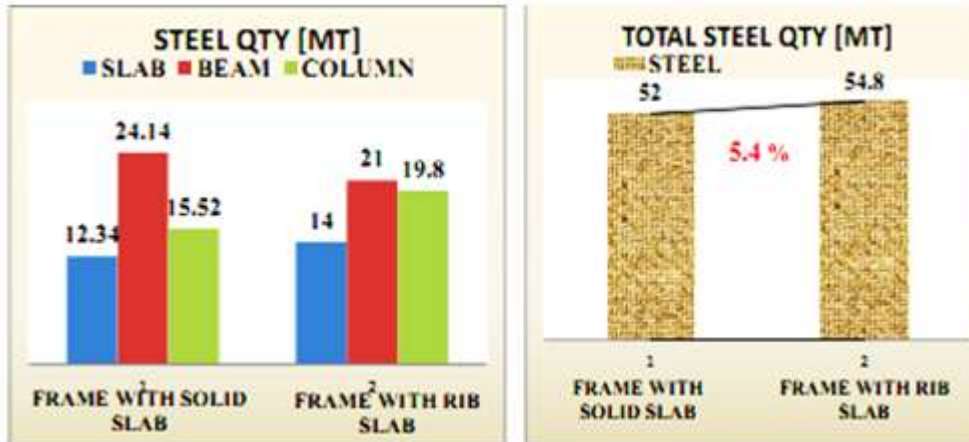
Figure 4. Steel Mass Comparison
